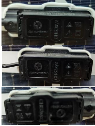
Fig. 5: detail view of closed junction box
